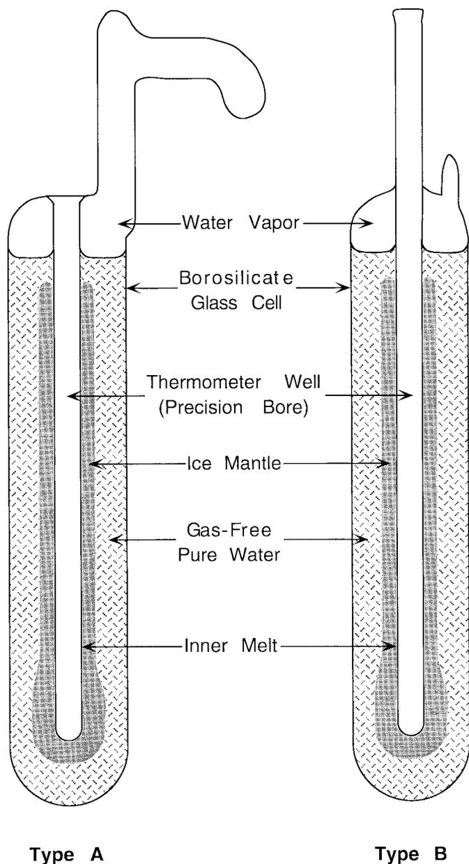
**FIG. 1 Configurations of two commonly used triple point of water cells, Type A and Type B, with ice mantle prepared for measurement at the ice/water equilibrium temperature. The cells are used immersed in an ice bath or water bath controlled close to 0.01°C (see 5.4)**
